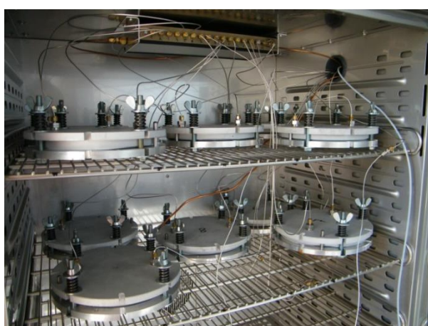
Figure 1: Measurement cells in climate chamber (exemplary layout)
