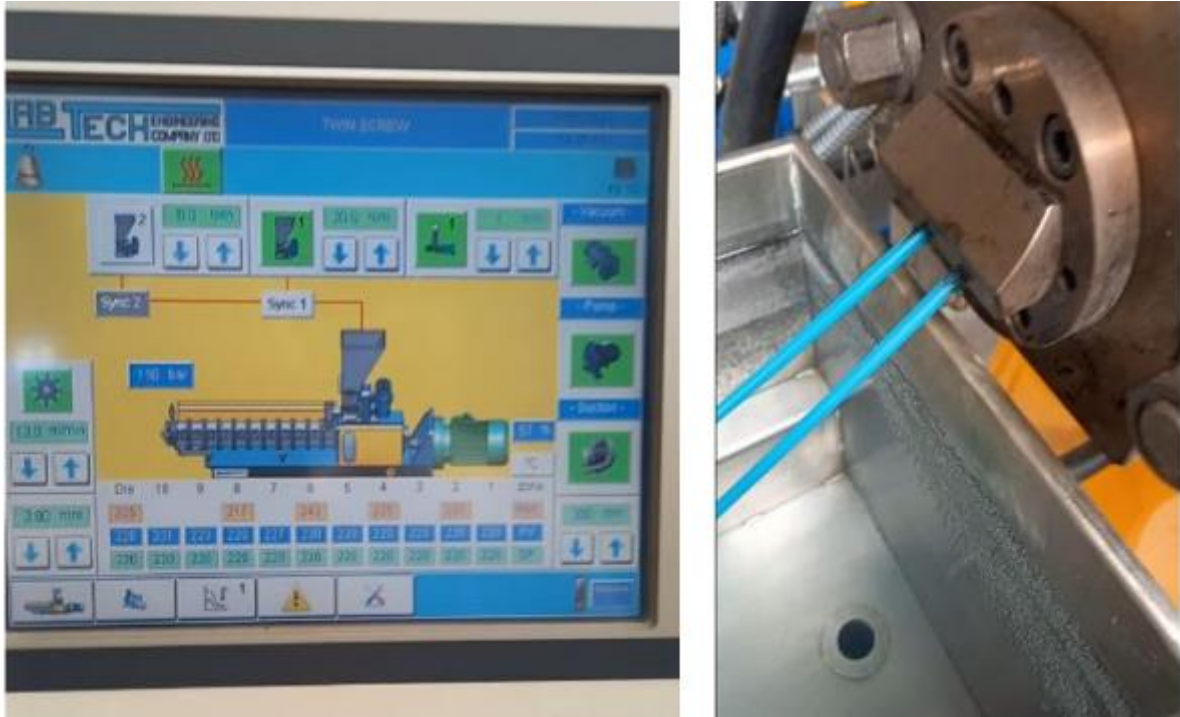
Figure 5: Operating settings and die exit of the Labtech extruder at SUEZ SA.
