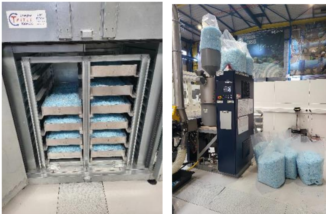
Figure 4a (left): overnight drying of flakes to reduce moisture content and 4b (right) Densifier Intarema 504K at SUEZ SA.
