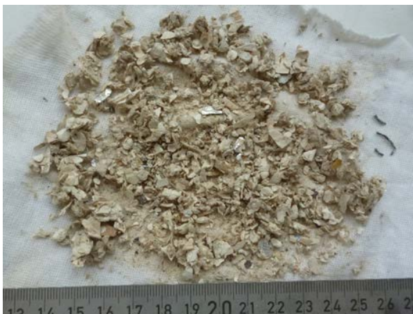
Figure 5: Residue after consecutive extraction of all polymers
