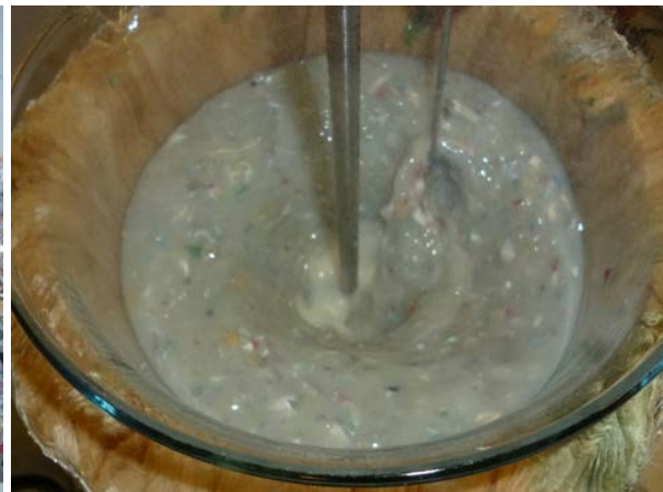
Figure 1: Flexible food packaging waste (FR) Figure 2: Dissolution of PE
