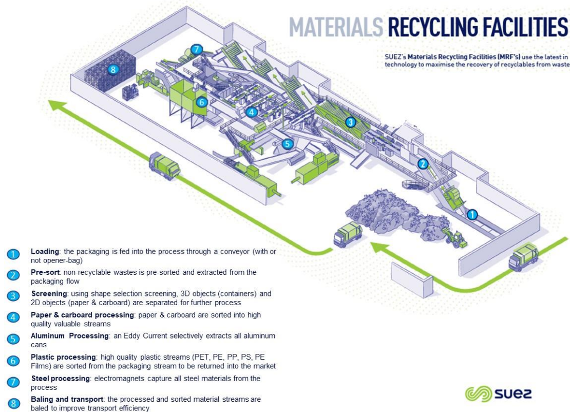
Figure 3: Typical process of Materials Recycling Facilities (SUEZ)
