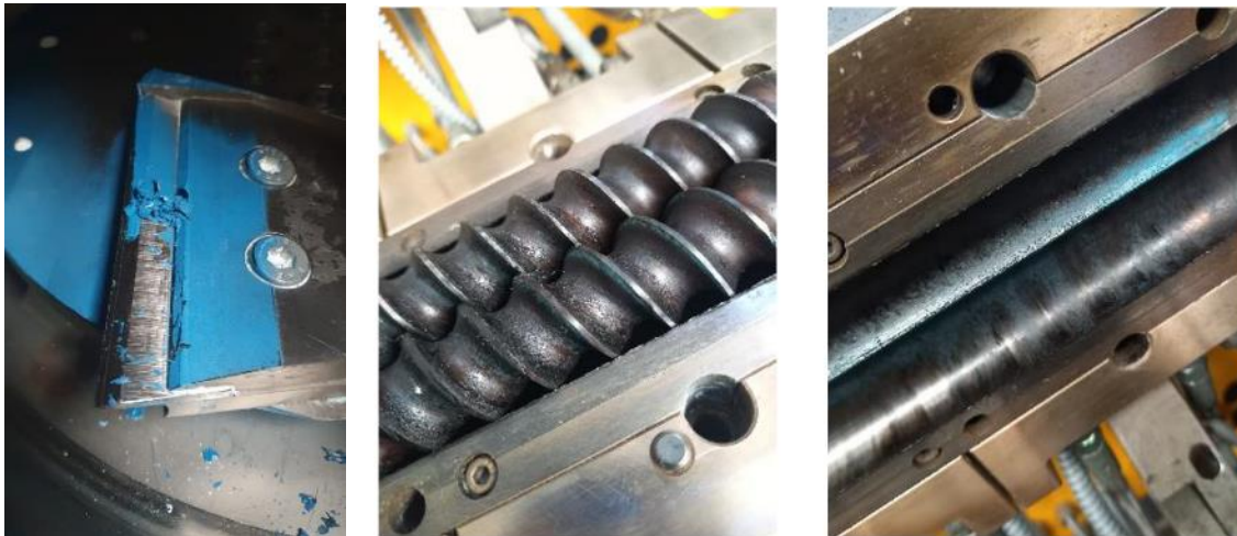
Figure 10a (left): significant blue colour deposition on the blades in the densifier and 10b (middle and right): minor blue residue on screws and shaft of extruder.
