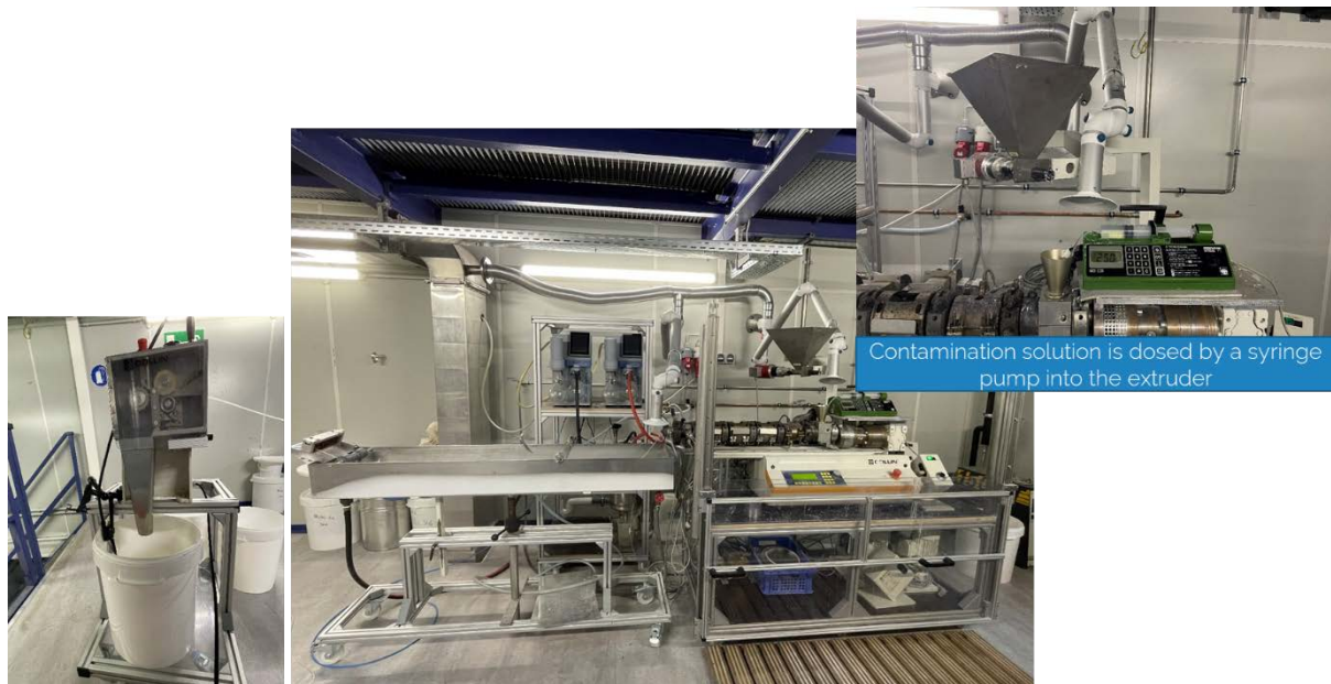
Figure 1: Contamination set-up at Fraunhofer IVV, from left to right: pelletizer, full extruder set-up with dry ice cooling bath, syringe system to pump the contamination solution into the extruder. The process flow starts with the dosing of the contamination solution, extrusion and then pelletizing.
