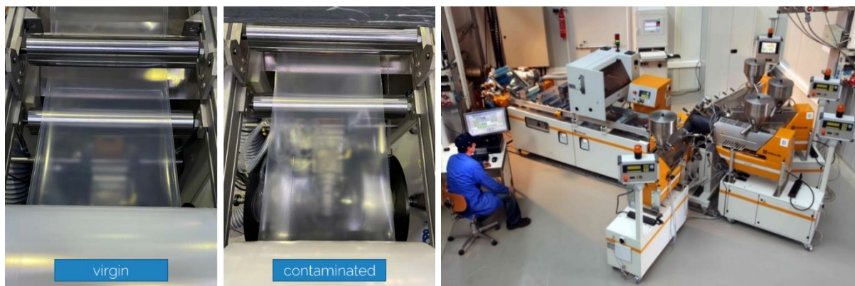
Figure 2: virgin (left) and contaminated (middle) PE film extruded at IVV on a Dr. Collin extruder (right)
