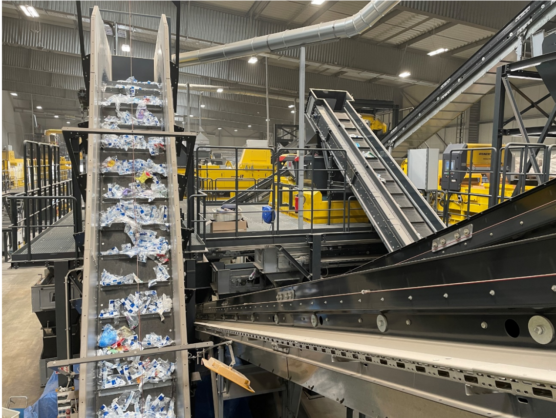
Figure 17: Sorting line in Steinert Sorting Center Pulheim with background waste and tracer-based pouches on the conveyor belt (the conveyor seen on the right side is not used during actual sorting. It can be used to circulate the material on the conveyor system to increase or decrease the belt coverage within the system)
