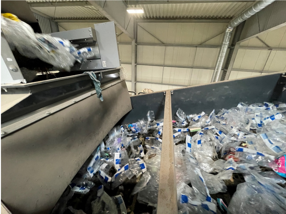
Figure 21: end of conveyor belt and ballistic separator with background waste and tracer-based pouches
