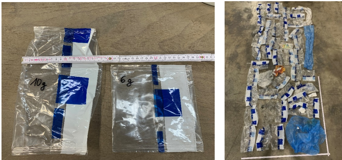
Figure 2 (left) single pouches (12.6 g and 6 g, nominally as produced) and (right) specific area weight measurement for drop of the first sorting step to determine the mass throughput values.
