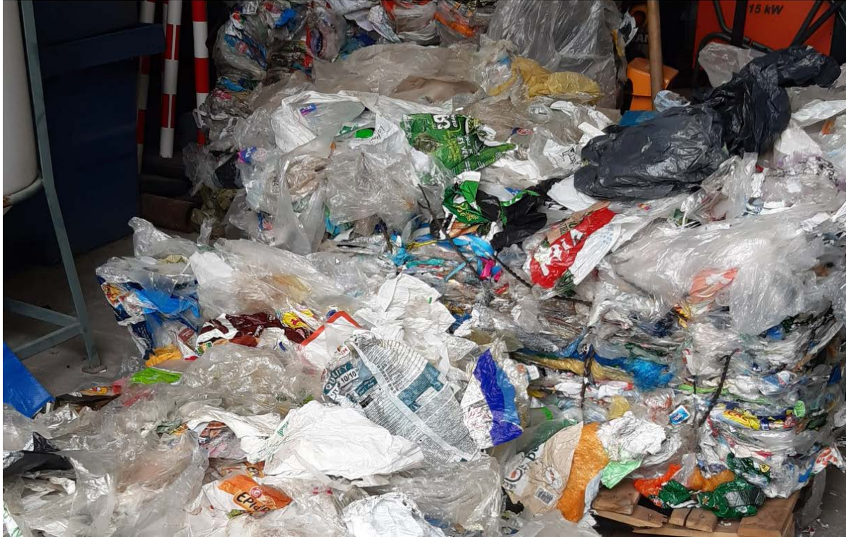
Figure 15: Decompressed bale of flexible French packaging waste used as background for sorting trials
