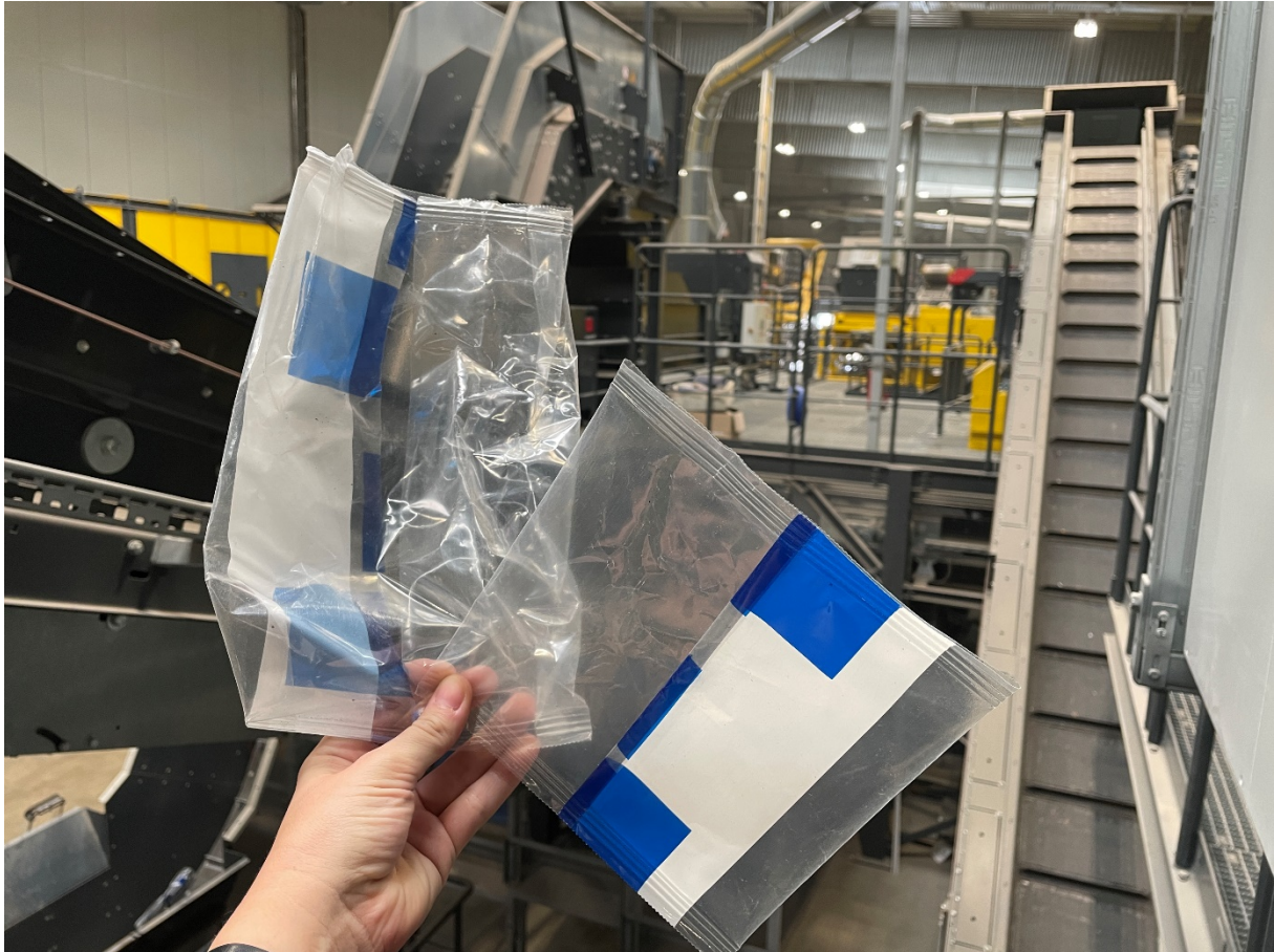
Figure 16: Tracer-based pouches in front of the sorting line in Steinert Sorting Center in Pulheim
