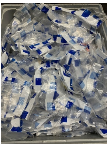
Figure 12 Final Product after Step 2: Cleaning. High purity in traced food-grade material achieved
