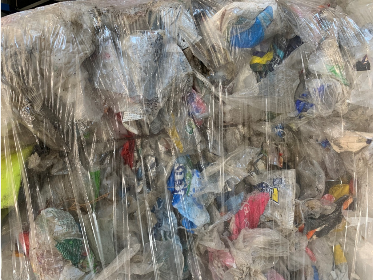
Figure 19: Bale with French post-consumer packaging waste used as background material for sorting trials, before opening the bales
